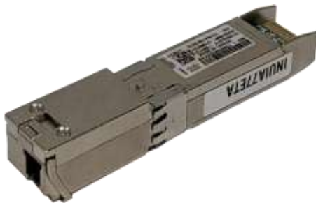
Figure 7. 10G Long-Reach (LR) BiDirectional Transceivers (Upstream and Downstream)
