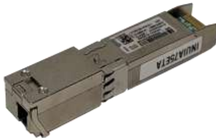
Figure 7. 10G Long-Reach (LR) BiDirectional Transceivers (Upstream and Downstream)
