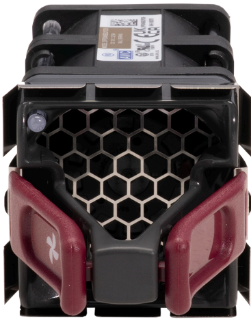
Figure 4. Field-replaceable fan units for 1RU models
