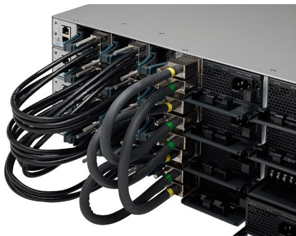
Figure 9. StackWise-480 and StackPower connectors
